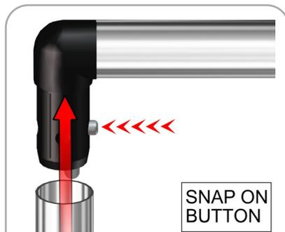
Connect bottom and top tubes to side tubes following the labels.
