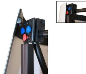
To attach panels, start with the left curved endcap panel, hook panel on blue button. Attach rest of panel to magnetic channel bar.
