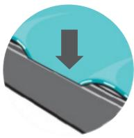
Fit graphic into corners, then "tap" into rest of frame channel.
